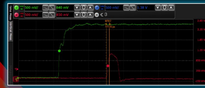
Fig 2. Controllable short beacon pulse with rise time of 777ps. The red pulse is the beacon optical pulse received by detector while the green one is the trigger signal. This is generated with the conditions of pulse width = 3.1ns, repetition = 100kHz, average transmit power = 34.7uW, attenuator = 40dB, expected received peak power = 8.9uW
